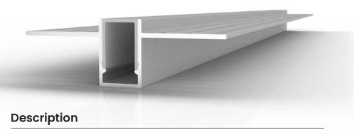
The Diffusion SLC-Micron-006T is a narrow 10 mm trimless anodized aluminum channel that comes complete with mounting hardware, end caps, and an opal polycarbonate lens for zero dotting and It offers lens options for both flush and regressed installations.
