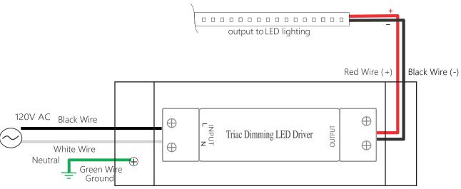
Green wire / Enclosure wire must be grounded
