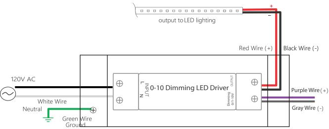
Green wire / Enclosure wire must be grounded
